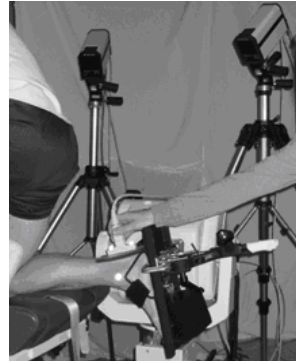
Figure 1. Subject placement in Biodex with markers and gel standoff pad attached. Ankle is in neutral angle with knee at 90°.
