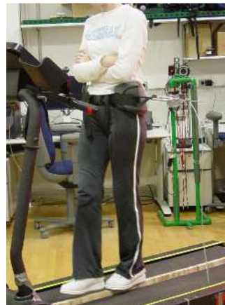
Figure 1. A subject walking on the beam-mill with a lateral assist device used to provide a restoring force towards the center of the beam.
